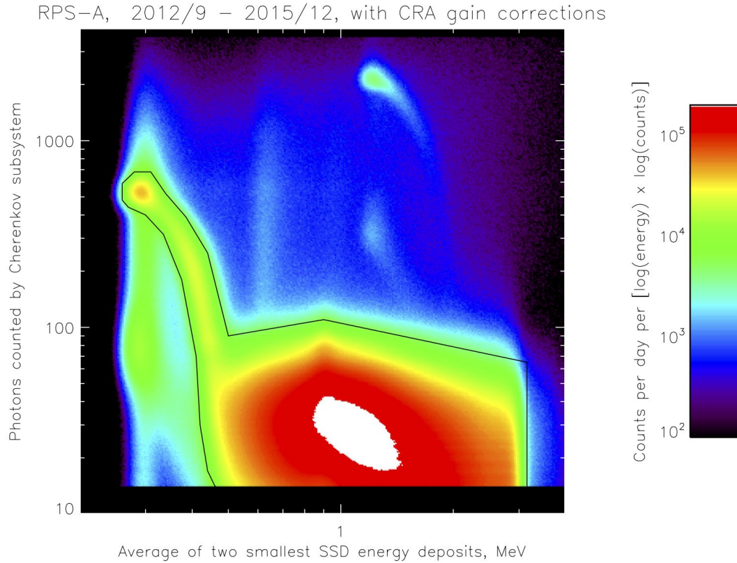
Figure 3. Cherenkov vs. MIN2SSD cuts, the so-called Nessie plot. These cuts remove high-energy particles and non-proton backgrounds. Points outside the polygon are considered backward or, at least, not forward.
